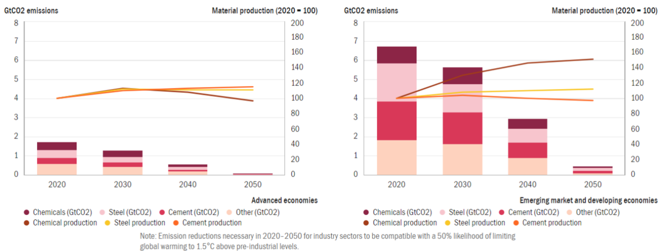
Figure 2: Speed of transition in difficult to abate sectors: cement and steel production
